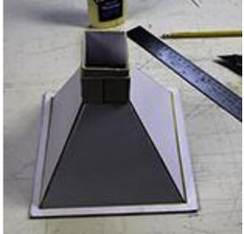
accessory flash. It is made from scrap pieces of mounting board and a piece of white fabric on the front that acts as a diffuser (no duct tape was used). Other diffusing materials could work as well but must be neutral in color so as not to effect color temperature (unless that's what you want to do. The opening for the
